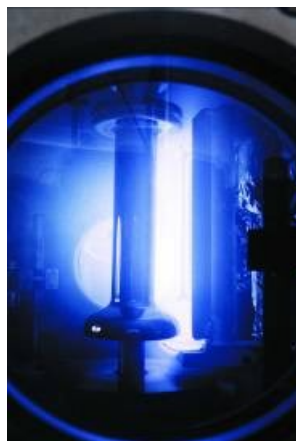
Thin films by sputtering or evaporation
