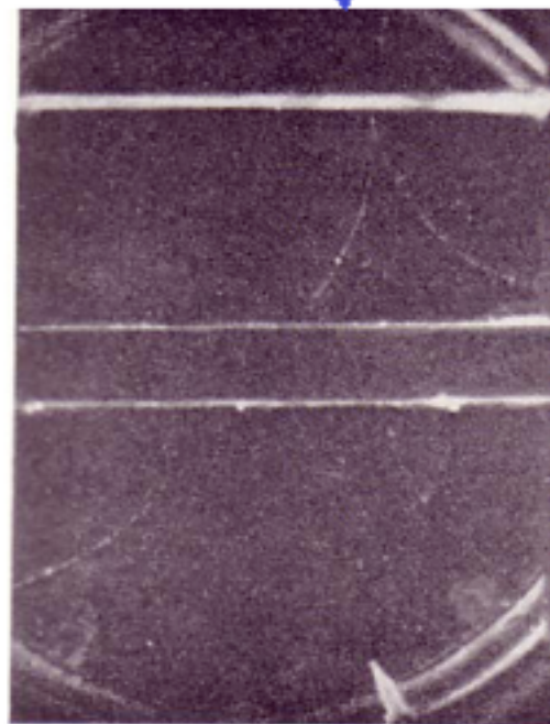
Production of an electron-positron pair by a high-energy photon in a Pb plate
