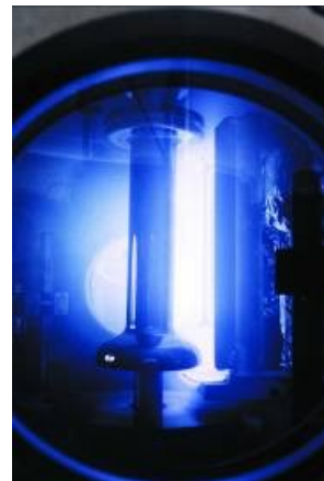
Thin films by sputtering or evaporation
