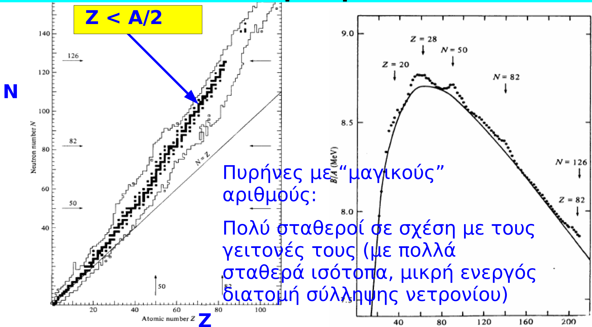
Fig. 4.6 The \beta -stability valley. Filled squares denote the stable nuclei and long-lived nuclei occurring in nature. Neighbouring nuclei are unstable. Those for which data on masses and mean lives are known fill the area bounded by the lines. For the most part these unstable nuclei have been made artificially. (Data taken from Chart of the Nuclides (1977), Schenectady: General Electric Company.)
