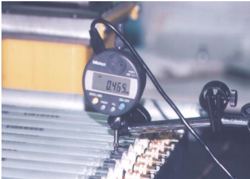
Figure 14: End-plug height measurements with the mechanical feeler (mitutoyo).
