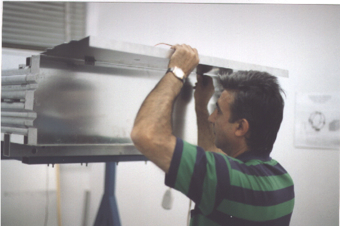
Figure 5: End face of the chamber showing the Faraday cage with its cover being opened. Note that in this position the chamber support is located below the chamber and the chamber is turned upside down compared to the sketch of Figure 1.
